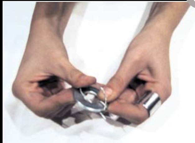
2 Twist it around one side of the washer. Tighten it with the wire cutter.
